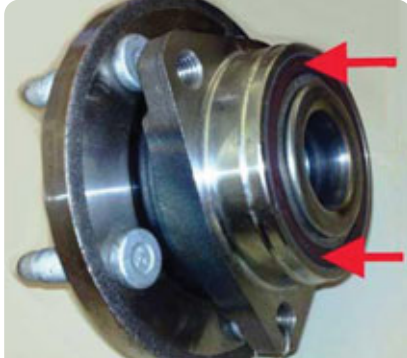
New bearing design with magnetized nitrile rubber ring
