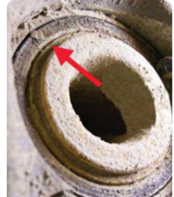
Typical debris on the magnetic encoder ring before cleaning
