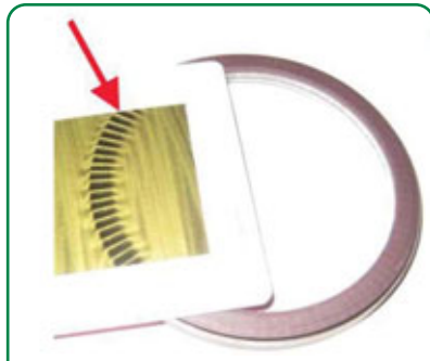
Magnetic encoder ring with North and South poles shown
